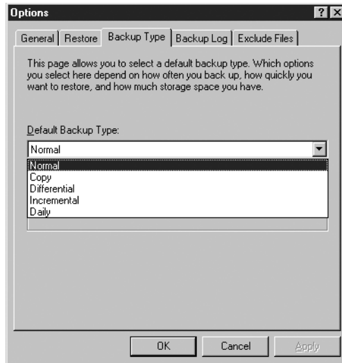
Figure 4-4 The Backup Type tab in the Windows Server 2003 Backup program's Options dialog box
